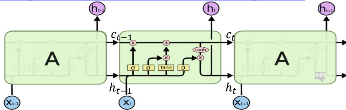
The repeating module in an LSTM contains four interacting layers.
